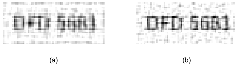
Figure 10: (a) TSVD with discrepancy principle with c=1.01 and \delta=0.01 \cdot \text{norm}(b) ( k=450 ); (b) TSVD with GCV ( k=576 );
