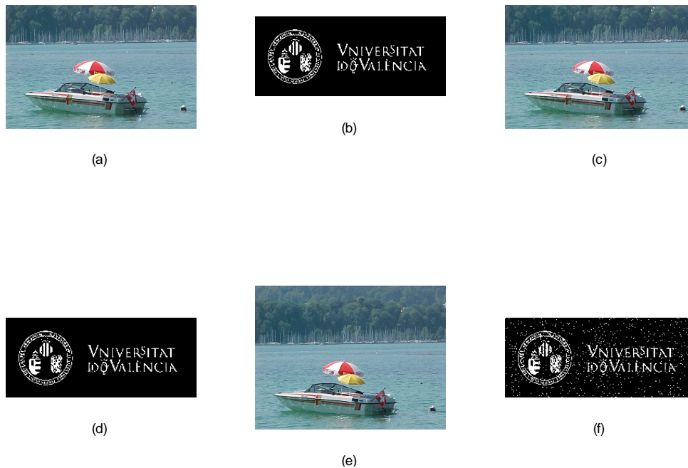
Figure 4: (a) Host image yacht; (b) Binary watermark; (c) Watermarked image; (d) Extracted watermark (correlation 1); (e) Watermarked image attacked with 2% additive Gaussian noise; (f) Extracted watermark from image (e) (correlation 0.8345).
